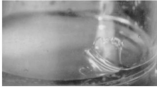
Figure 10.11: An acoustically induced liquid sheet in a cylindrical cavity by an acoustic mode with two nodal diametrical planes.
